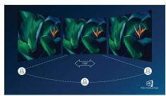
IPS displays use an advanced technology which gives you extra wide viewing angles of 178/178 degree, making it possible to view the display from almost any angle - even in 90 degree Pivot mode! Unlike standard TN panels, IPS displays gives you remarkably crisp images with vivid colors, making it ideal not only for Photos,
