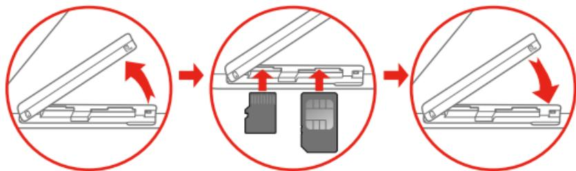
**Step 1.** Open the card slot cover as shown.
