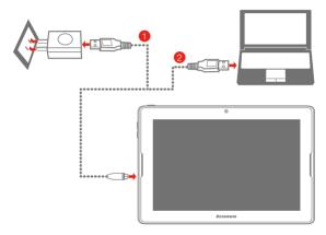
Method 1. Connect your tablet to a power outlet using the included cable and USB power adapter.
