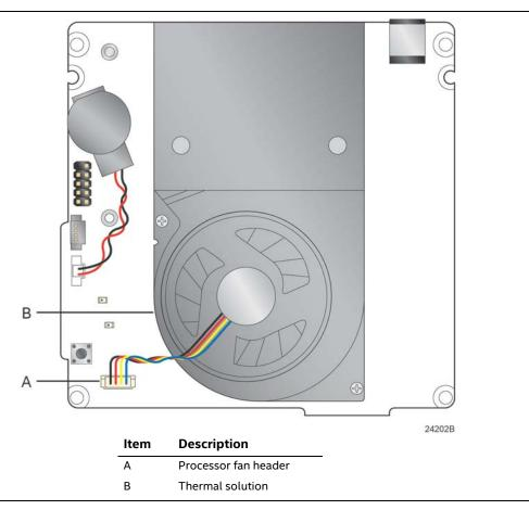
Figure 7. Thermal Solution and Fan Header
