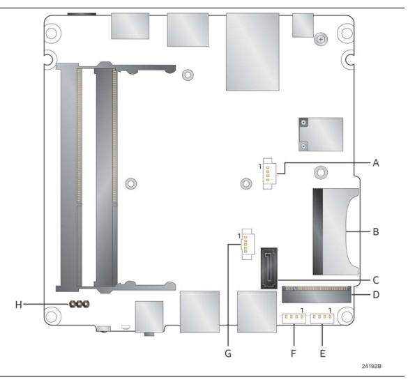
Figure 12. Connectors and Headers (Bottom)
