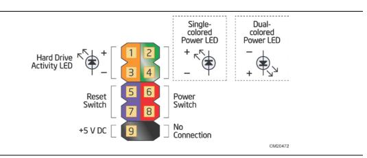
Figure 13. Connection Diagram for Front Panel Header (2.0 mm Pitch)
