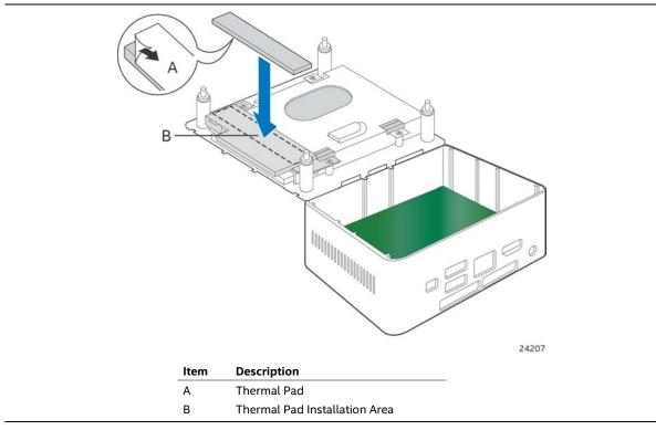
Figure 21. Installation area of Thermal Pad for Intel NUC Kit NUC6i5SYH/NUC6i3SYH
