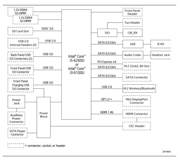
Figure 3. Block Diagram
