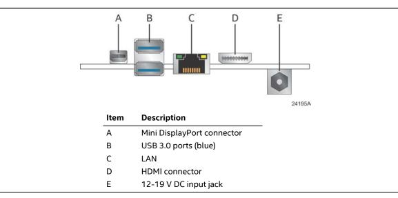
Figure 10. Back Panel Connectors
