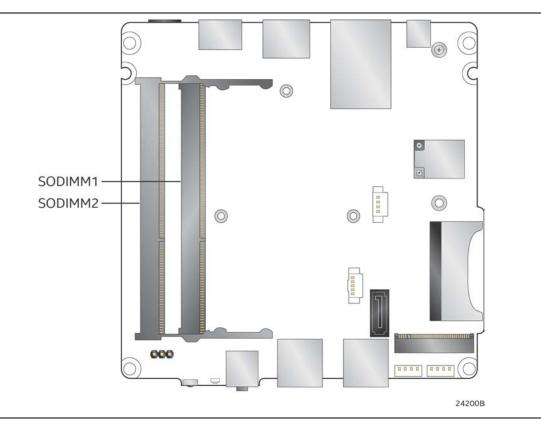
Figure 4 illustrates the memory channel and SO-DIMM configuration.
