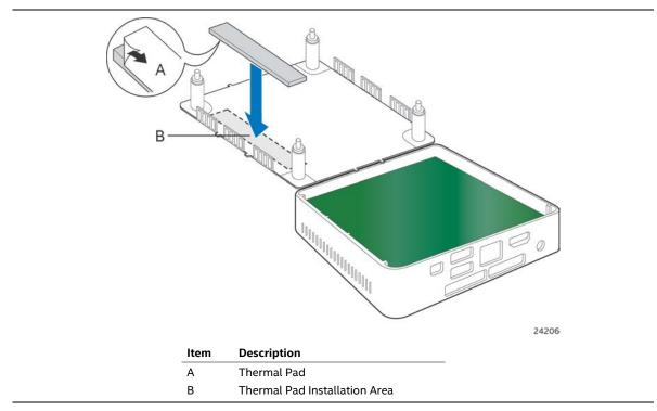
Figure 20. Installation Area of Thermal Pad for Intel NUC Kit NUC6i5SYK/NUC6i3SYK
