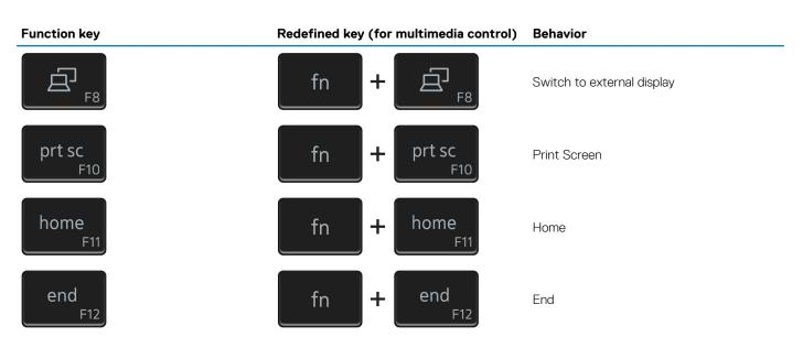
The **Fn** key is also used with selected keys on the keyboard to invoke other secondary functions.
