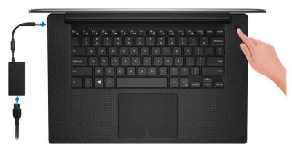
INOTE: To conserve battery power, the computer might enter into power save mode. Connect the power adapter and press the power button to turn on the computer.
