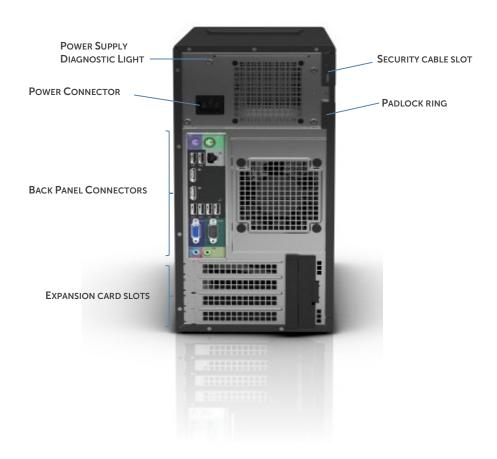
Figure 2. Back panel view and features
