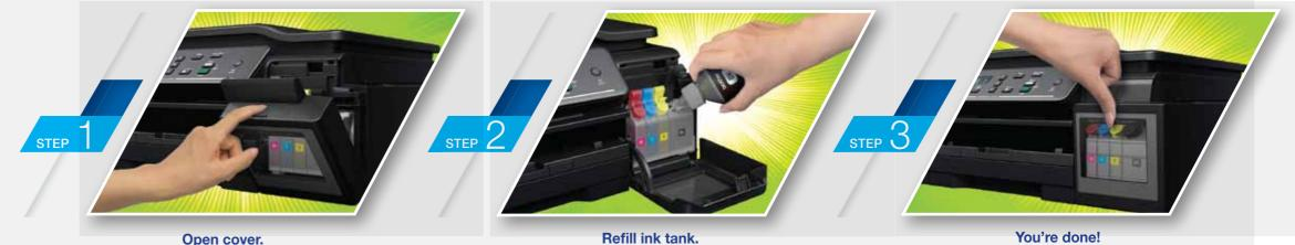
Remove tank cap. Tilt ink bottle at 45° angle
