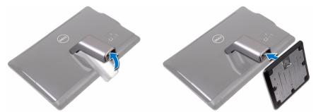
b) Tighten the captive screw to secure the base to the stand riser.
