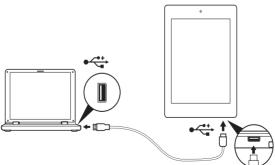
Using the micro USB to USB cable, connect the micro end into your tablet and the other end into your computer.
